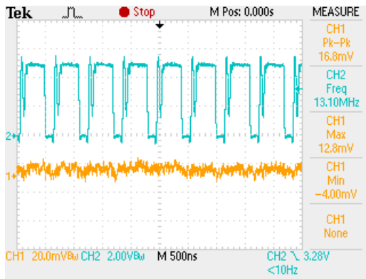
STEADY STATE OPERATION (VIN=5V, VOUT=3.3V, IOUT=100mA)
