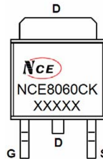
Marking and pin assignment
