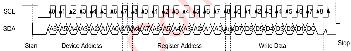
Fig 27 I 2 C Write Timing
