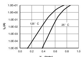
V<sub>SD</sub> (Volts) Figure 6: Body-Diode Characteristics (Note E)
