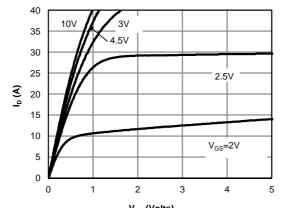
$V_{DS}$  (Volts) Fig 1: On-Region Characteristics (Note E)
