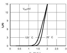
V<sub>GS</sub>(Volts) Figure 2: Transfer Characteristics (Note E)
