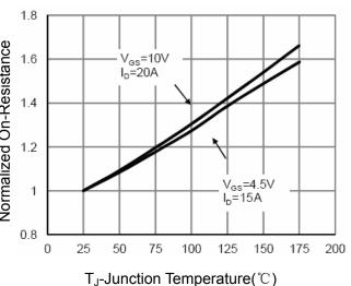
**Figure 4 Rdson-Junction Temperature**
