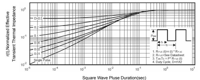
Figure 11 Normalized Maximum Transient Thermal Impedance
