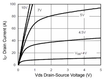
**Figure 1 Output Characteristics**
