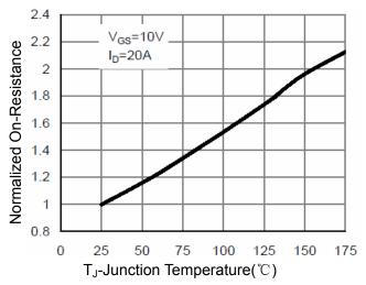
**Figure 4 Rdson-Junction Temperature**
