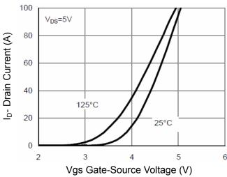
**Figure 2 Transfer Characteristics**
