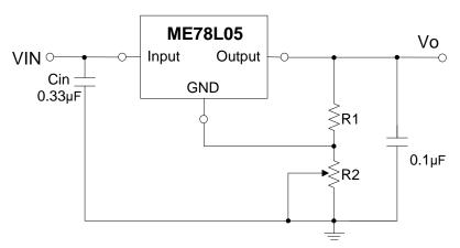
Fig.3 Adjustable Output Regulator
