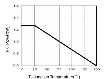
Figure 3 Power Dissipation
