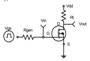
**Figure 1:Switching Test Circuit**
