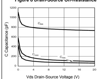
Figure 10 Capacitance vs Vds
