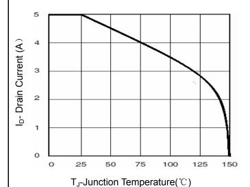
**Figure 4 Drain Current**
