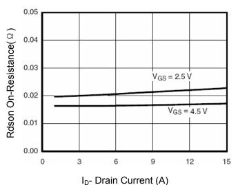
Figure 6 Drain-Source On-Resistance
