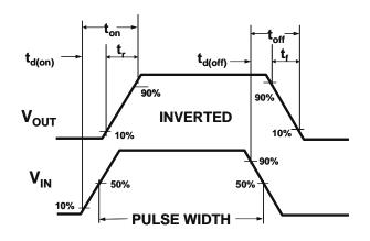
Figure 2:Switching Waveforms
