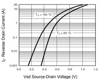
Figure 12 Source- Drain Diode Forward
