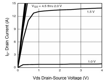
**Figure 5 Output Characteristics**
