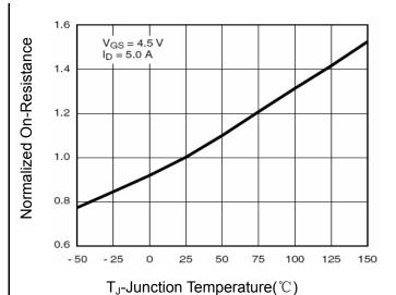
Figure 8 Drain-Source On-Resistance
