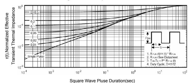
**Figure 14 Normalized Maximum Transient Thermal Impedance**
