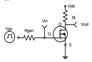
**Figure 1:Switching Test Circuit**
