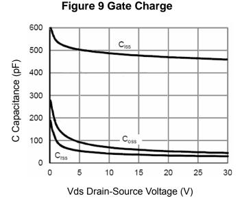
Figure 11 Capacitance vs Vds
