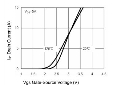
**Figure 4 Transfer Characteristics**
