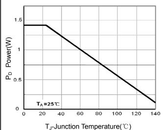
Figure 8 Power Dissipation
