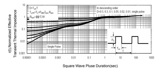
**Figure 13 Normalized Maximum Transient Thermal Impedance**
