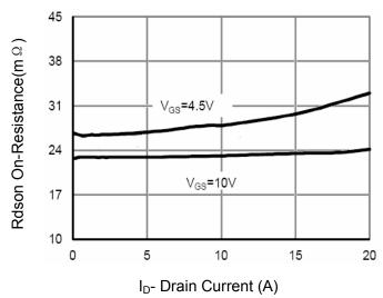
Figure 5 Drain-Source On-Resistance
