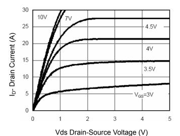
**Figure 3 Output Characteristics**
