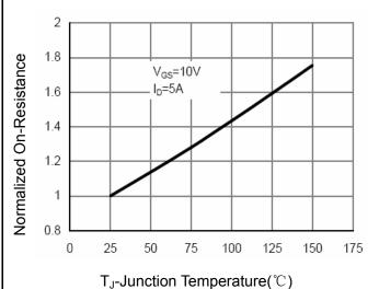
Figure 6 Drain-Source On-Resistance
