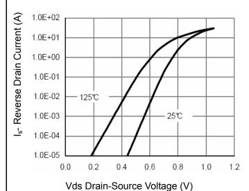
Figure 10 Source- Drain Diode Forward
