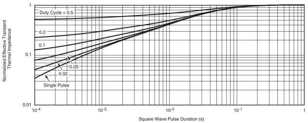
Normalized Thermal Transient Impedance, Junction-to-Foot
