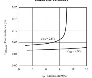
On-Resistance vs. Drain Current and Gate Voltage
