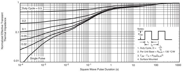
Normalized Thermal Transient Impedance, Junction-to-Ambient
