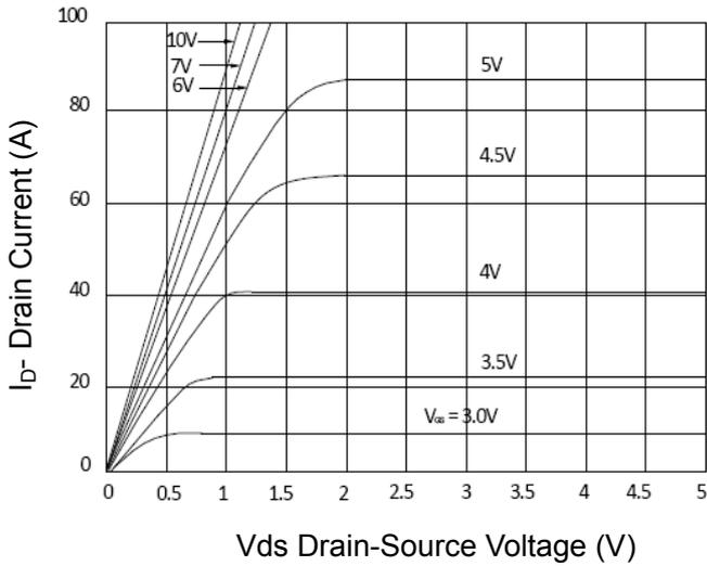
**Figure 1 Output Characteristics**
