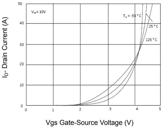
**Figure 2 Transfer Characteristics**
