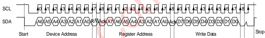
Fig 24 I 2 C Write Timing
